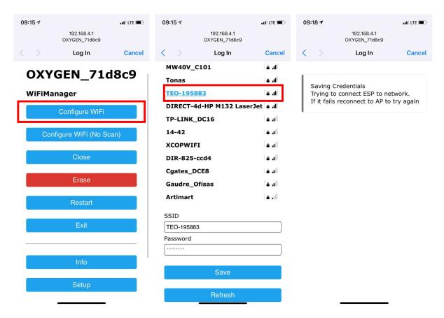
Figure 12. WiFi connection set-up
