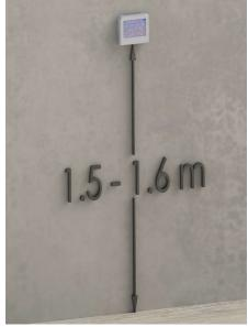
Figure 6. Installation of the control panel
