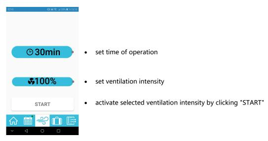
Figure 16. Ventilation boost activation
