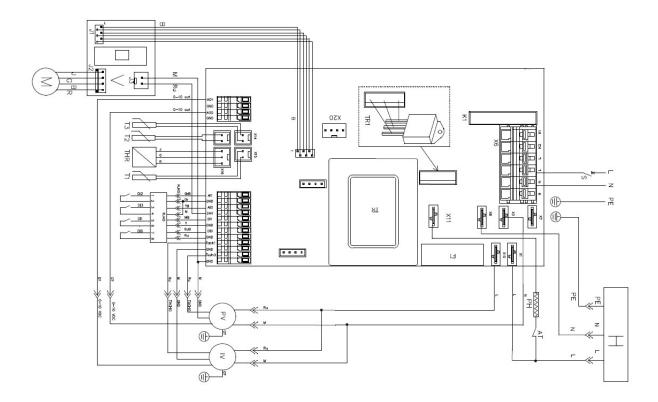
Figure 10. Control board electrical wiring diagram
