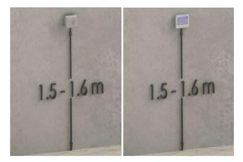
Figure 7. Installation of the control panel
