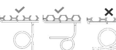
**Before starting the unit for the first time or after a longer standstill, check the water trap. If you make a bend on the hose, pay attention to the correct bend radius to avoid "breaking the hose". To extend the siphon hose, always choose a hose - pipe of the same or larger diameter. Always choose the hose-pipe coupling with the smallest reduction of the inner diameter.**
